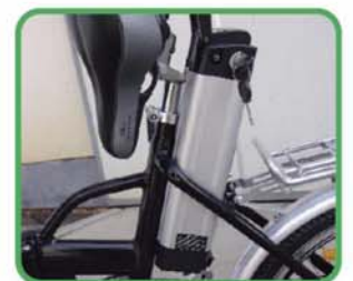
Lithium battery, comes with keyed security lock and flip seat for easy battery removal
